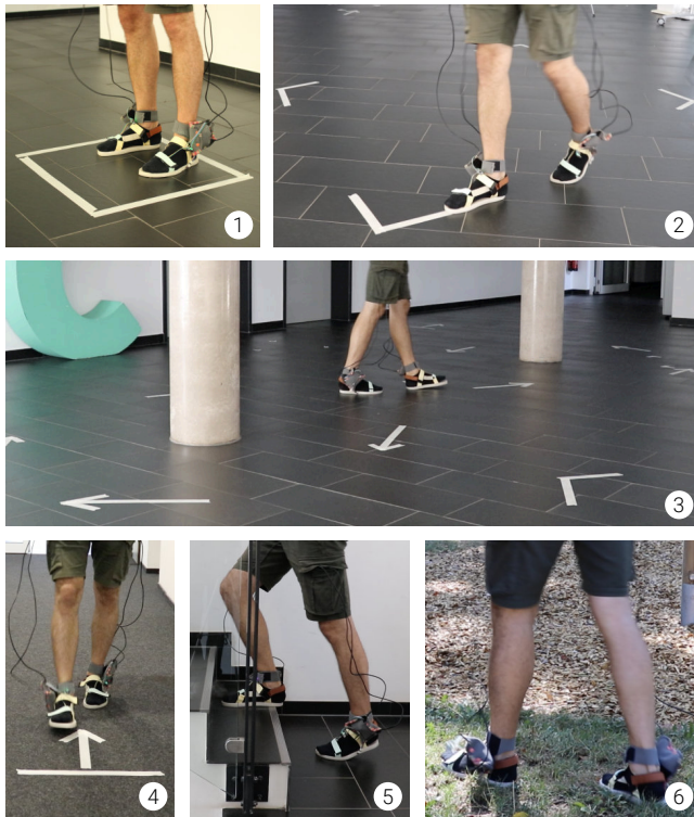
Figure 8: Exploring vibrotactile augmentation indoors and outdoors: (1) exploring the augmentation while standing and shifting the center of mass in a small area, (2) walking along a 3 by 3 meter square, (3) walking an eight-shape between two piles, (4) walking a hallway on two different surfaces (stone and carpet), (5) walking up and down stairs, and (6) walking outside on grass and wood chips.
