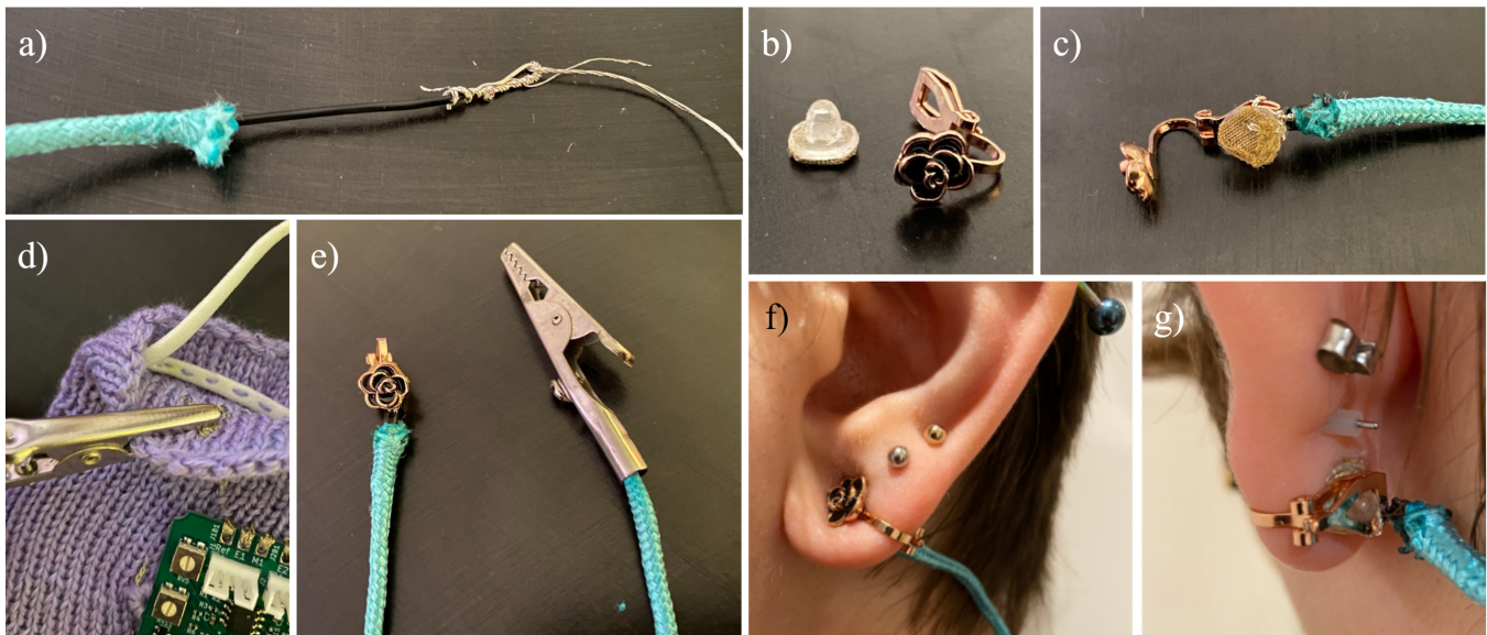
Figure 9: The construction of the earring reference electrode, starting with the cabling (a), stitching the conductive fabric to the earring pad (b-c), and securing the electrode to the collar and reference inputs (d) for a complete wearable (e). Reed wears the the electrode as part of their normal jewelry (f, g).
