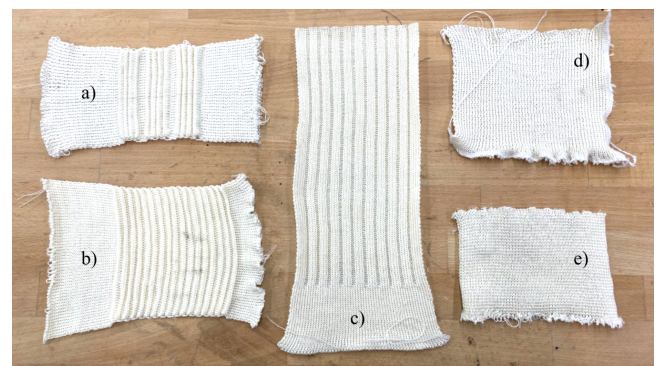
Figure 3: Samples of different knit structures for the collar body. Three Milano rib variations (a, b) were compared to a 2x3 rib (c) and two full bed rib stitches (d, e).
