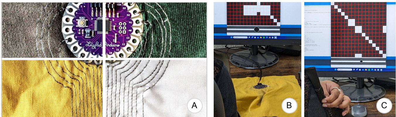
Figure 1: Recreating an eTextile sensor, Pinstripe , on four different fabric swatches (A) for tabletop (B) and wearable (C) pinch and rolling gestures.
